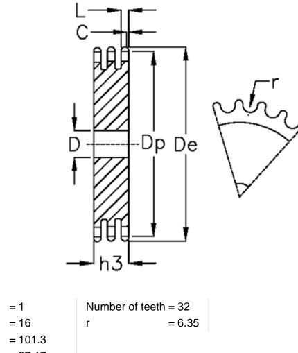
C = 1 D = 16 De = 101.3 Dp = 97.17 For chain size =  $3/8 \times 7/32$ For chain type = 06 B-3 h3 = 25.6 L = 5.2
